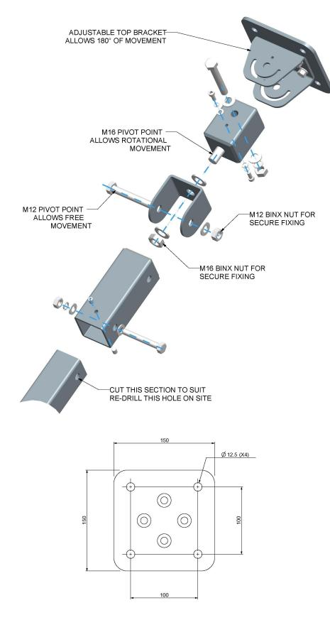
Drillings for Top Plate fixing. Nominal Hole size is 12.5mm for 12mm fixings. The top fixing plate is 6 mm thick mild steel plate, the pivot saddle bracket is 4 mm thick mild steel plate. The top joint section is 60 X 60 X 4 SHS and the free movement pivot is also 4mm thick mild steel plate. The drop section is 50 X 50 X 4 SHS and fits inside the 60 X 60 X 4 SHS top joint section. The bottom plate is 6 mm thick mild steel plate.
