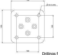
Drillings for Top Plate fixing. Nominal Hole size is 12.5mm for 12mm fixings. Our latest version of the Adjustable Drop VEID Bracket Assembly is designed to interface with the Infotec FM range of Video Displays (LED) FM42W and FM52W
