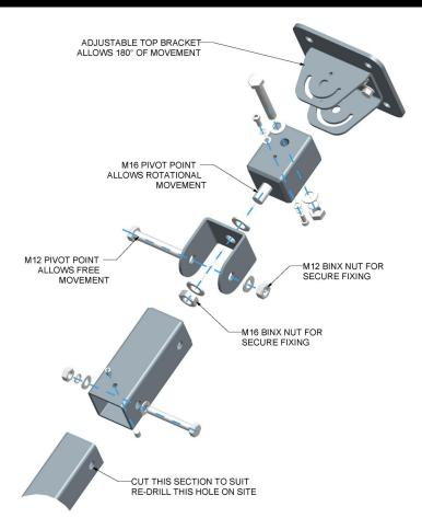
The top fixing plate is 6 mm thick mild steel plate, the pivot saddle bracket is 4 mm thick mild steel plate. The top joint section is 60 X 60 X 4 SHS and the free movement pivot is also 4mm thick mild steel plate. The drop section is 50 X 50 X 4 SHS and fits inside the 60 X 60 X 4 SHS top joint section. The bottom plate is 6 mm thick mild steel plate.
