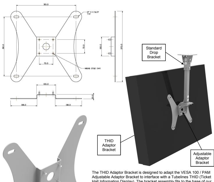
Hall Information Display). The bracket assembly fits to the base of our Standard Drop Brackets either Part No.151105-501 for the 1 metre long bracket or Part No.151105-601 for the 2 metre long bracket.
