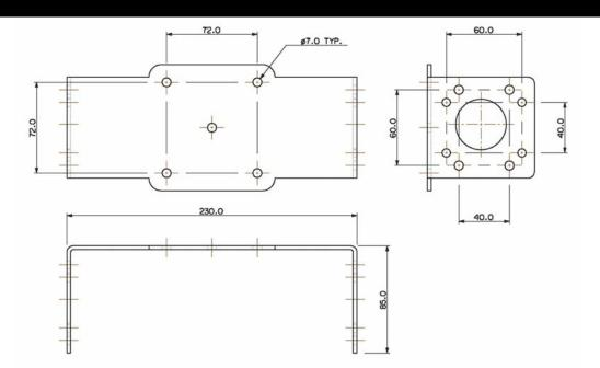
The Double Column Speaker Bracket has a gross weight of 0.76 Kilograms and is designed to mount Penton (or equivalent) column speakers to the base of our Standard Drop Brackets either Part No.151105-501 for the 1 metre long bracket or Part No.151105-601 for the 2 metre long bracket.
