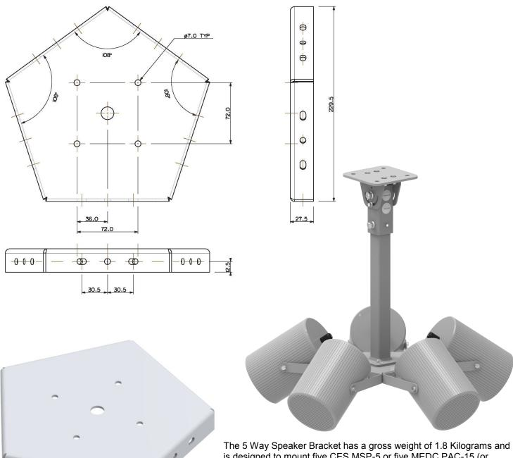
The 5 Way Speaker Bracket has a gross weight of 1.8 Kilograms and is designed to mount five CES MSP-5 or five MEDC PAC-15 (or equivalent) speakers to the base of our Standard Drop Brackets either Part No.151105-501 for the 1 metre long bracket or Part No.151105-601 for the 2 metre long bracket.
