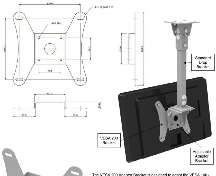
The VESA 200 Adaptor Bracket is designed to adapt the VESA 100 / PAM Adjustable Adaptor Bracket to a full VESA 200 compliant configuration. The bracket assembly fits to the base of our Standard Drop Brackets either Part No.151105-501 for the 1 metre long bracket or Part No.151105-601 for the 2 metre long bracket.
