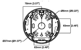
The AXIS Camera Adaptor Bracket has a gross weight of 0.9 Kilograms and is designed to mount the AXIS Dome Camera by means of the T94H01P Conduit back box (Supplied by AXIS) to the base of our Standard Drop Brackets either Part No.151105-501 for the 1 metre long bracket or Part No.151105-601 for the 2 metre long bracket.
