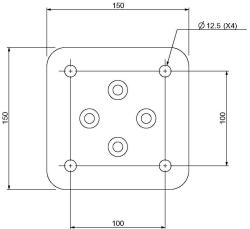
Drillings for Top Plate fixing. Nominal Hole size is 12.5mm for 12mm fixings.
