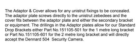
The adaptor plate weighs approx. 1.8 Kilograms and the aluminium cover 0.43 Kg and are attached with suitable fixings. We would suggest bright zinc plated 8.8 grade fixings in all cases and suitable single coil or Shakeproof washers.
